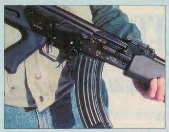
(above) Here the VEPR is seen with its safety/dust cover in the up, or ON position. Note the well-proportioned "beaver tail" style handguard. (right) Although it appears to be separate, the wellproportioned pistol grip of the VEPR is part of the butt stock.
